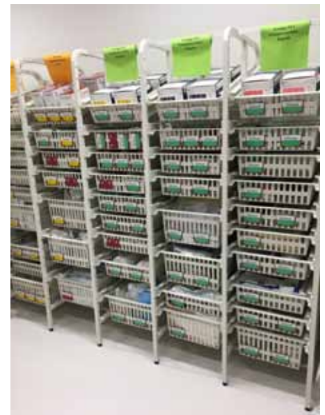
High density racks incorporated clipped on label holders
